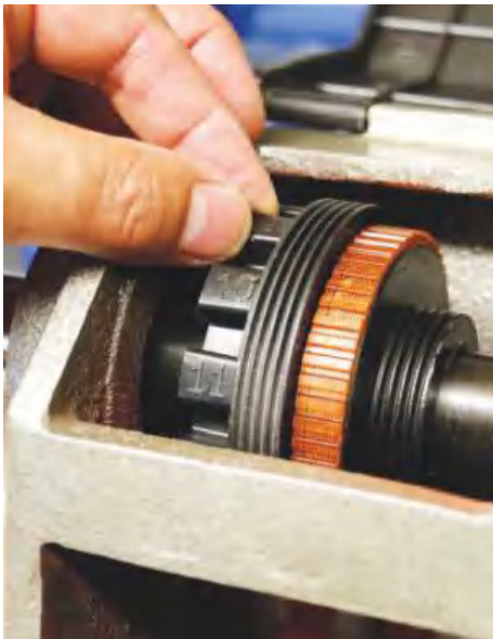
▲ The top pulley has 12 indexing positions
